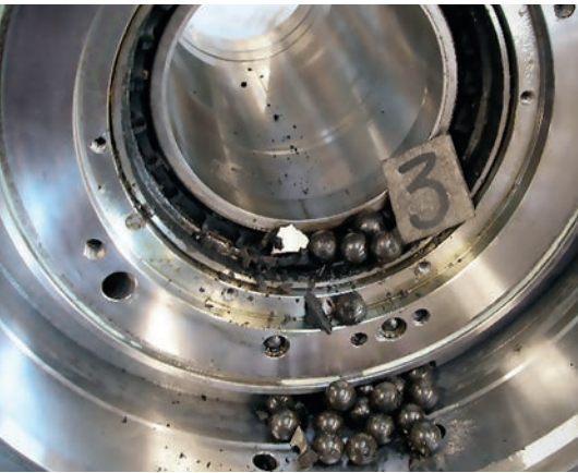
Spindle failure: A hazard for personnel and machinery
