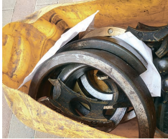
This counterfeit bearing caused major damage to a water desalination plant in the Mediterranean region
